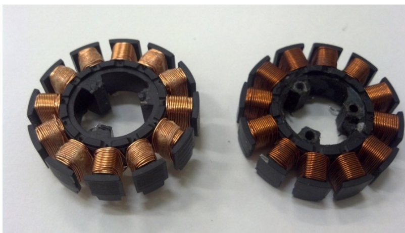
Fig. 5. Maxon burned winding, also without attachment holes (left) and our handmade winding with attachment holes (right).
