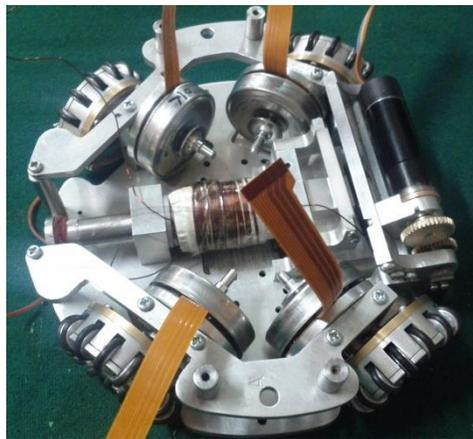
**Fig.2.4 (a) Top view of the kicker module showing the solenoid gun**
