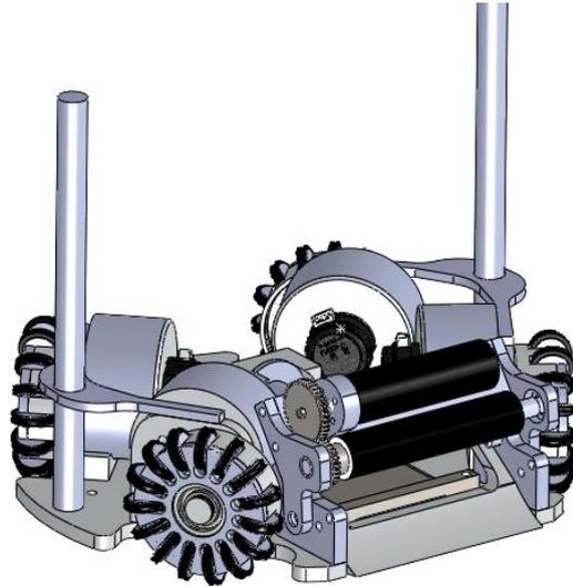
**Fig. 5.** Robot 2011 mechanical structure
