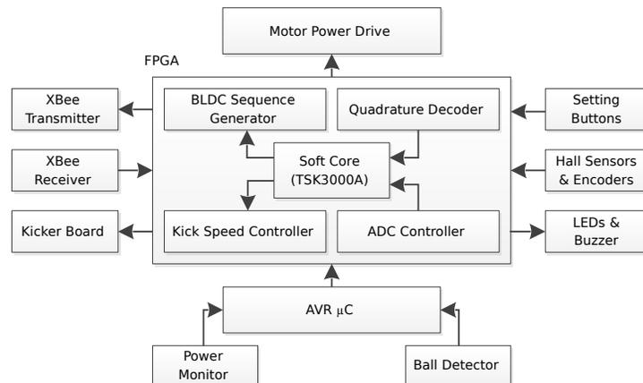
Fig. 7. The electrical system's diagram
