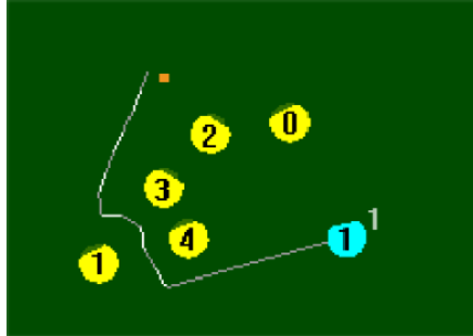
Fig. 7.1 Path generate by RRT algorithm
