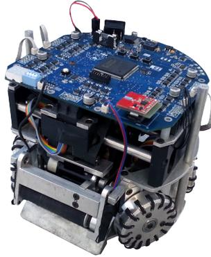
**Fig. 2.** The RoboFEI robot.
