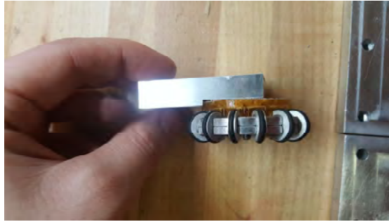
Fig. 5. View of the omni wheel-gear assembly.
