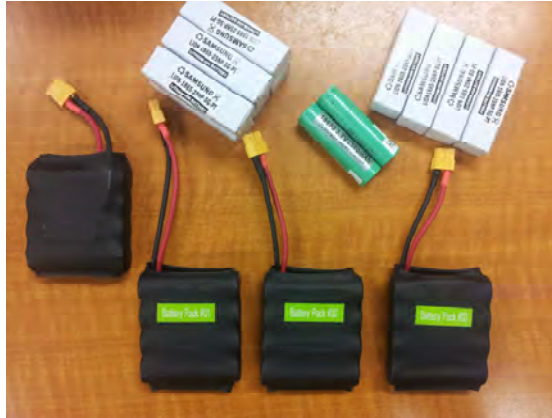
Fig. 9. Battery pack assembly beside individual cells
