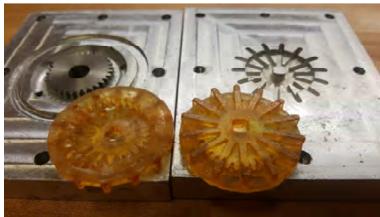
Fig. 4. View of the mold used to craft the internal gears.
