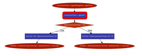
Fig. 3. Flow-chart of calculating desired deceleration
