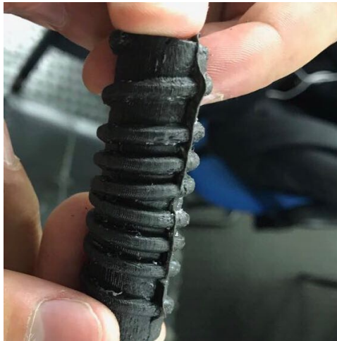
Fig. 8: Roller made with silicon rubber
