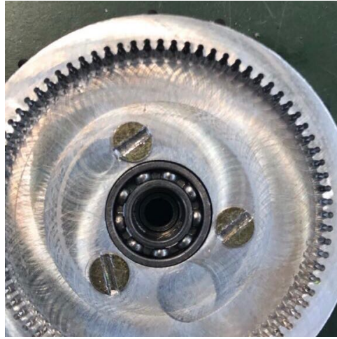
Fig. 6: The machined metal gear.
