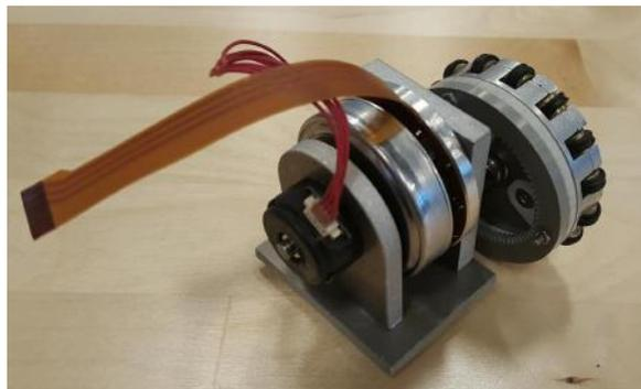
Fig. 2.6: Redesigned wheel mounted on a temporary baseplate
