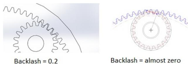
**Fig. 10.** old gearbox against new gearbox
