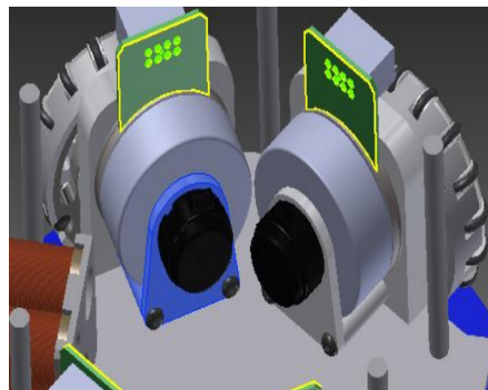
Fig. 5. Final geometry of the encoder support in blue.
