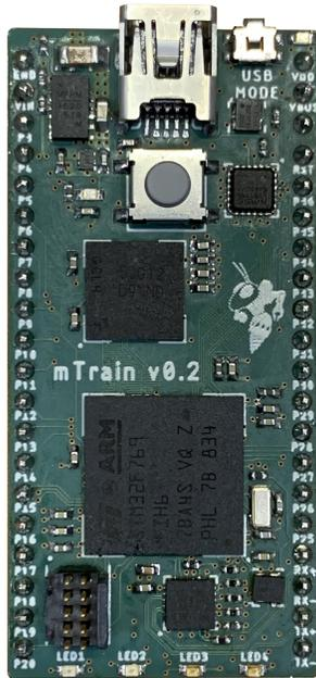
Fig. 6: Top view of new microcontroller board
