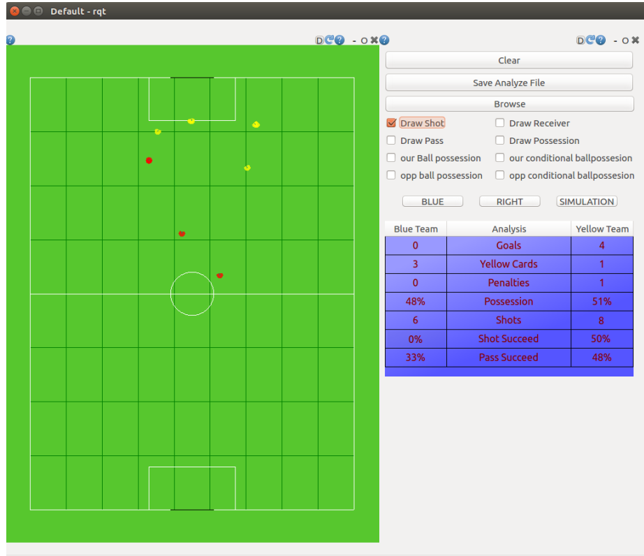
Fig. 20. The shot analysis obtained from a part of a game: yellow robots show the successful ones and red robots represents the failed shots. It can be understood that the shots in a nearer distance to the goal are more probable to be succeeded.
