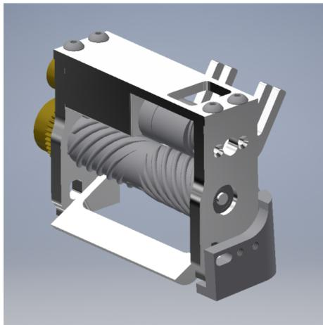
Fig. 4: Side view of the dribbler assembly
