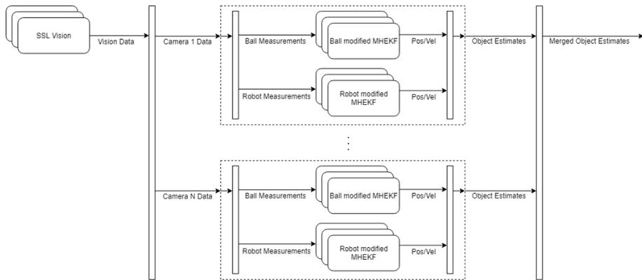
Fig. 9: Data flow from SSL Vision to final object estimate
