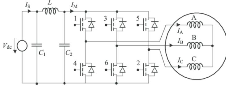
Fig. 18: A Circuit Diagram of a BLDC Motor [5]
