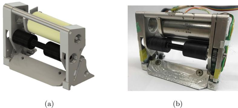
**Fig. 3.** Proposed dribbler (a)3D CAD image and (b)photo
