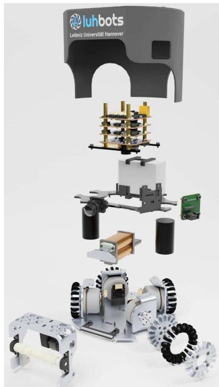
Fig. 2: Assembly of the first robot generation
