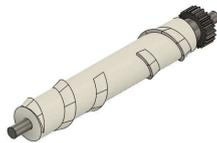
Fig. 7: Current design of the dribbler roller
