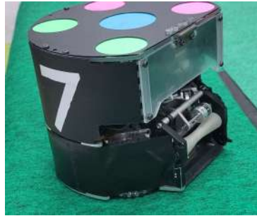
Fig. 7. Omni Wheel fixation
