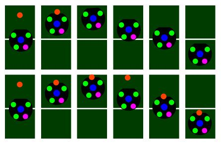
Fig. 8: Ball tracking during ball placement. In the upper row, the previous tracking with the regular Kalman filter is shown. In the lower row, the improved filter with dribbling support is used.
