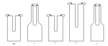
Fig. 3: Various plungers for test purposes: Plungers number 1, 2 and 3 are 3.2 mm wider than the old plunger and plunger number 4.
