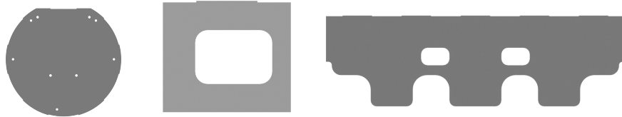
Fig. 2: The top, front and side part of our cover in order from left to right as they are cut out by the laser
