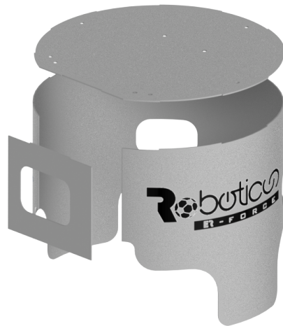
Fig. 3: Exploded view of the cover
