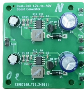
Fig. 9: First Prototype of Kicker Circuit
