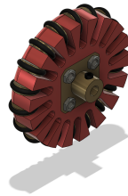
Fig. 2: Assembly behind the wheel with the coupling.
