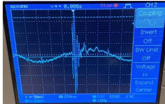
**Fig. 10.** 5V Ringing with GND as Reference During a Kick With  $2\Omega$   $1.5\text{nF}$  Snubber Added
