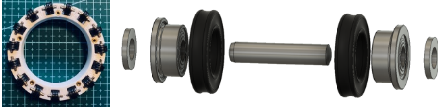
Fig. 3: Left: Subwheels mounted on PETG wheel chassis. Right: Subwheel exploded view, with washers, MF52 2Z bearings, NBR 4.47 mm \times 1.78 mm X-ring, 2 mm \times 10 mm dowel pin.
