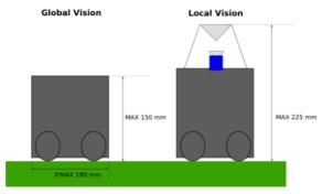
Figure 3: The maximum robot dimensions
