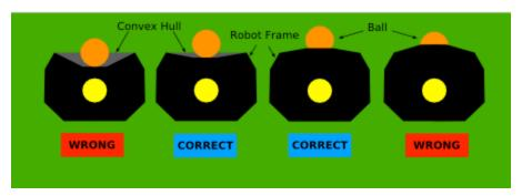
Figure 5: The 80/20 ball covering/holding rule
