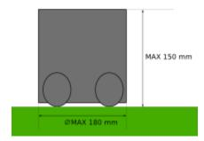
Figure 3: The maximum robot dimensions
