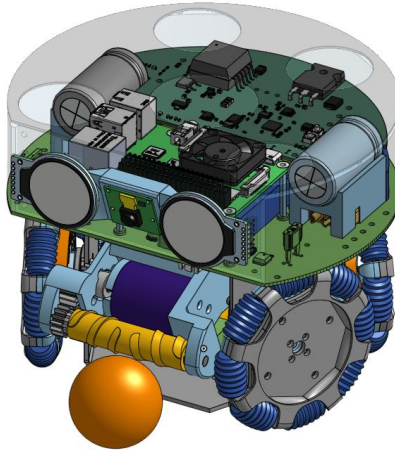
Fig. 1: CAD of Generation 1 Robot. Shell and faceplate are transparent for internal view.
