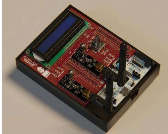
Fig. 4: A rendered image of the Transceiver Station v2 designed in Altium Designer.
