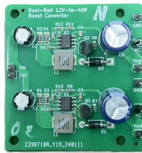
Fig. 9: First Prototype of Kicker Circuit
