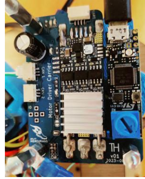
(b) With motor driver soldered in
