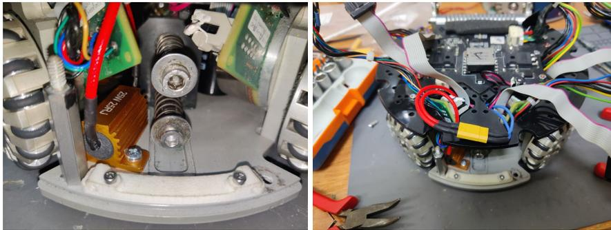
**Fig. 4.** Discharge resistor bolted to the aluminum plate and connected to the kicker PCB
