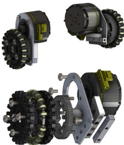
**Fig. 2.** Exploded view of the wheel actuator assembly
