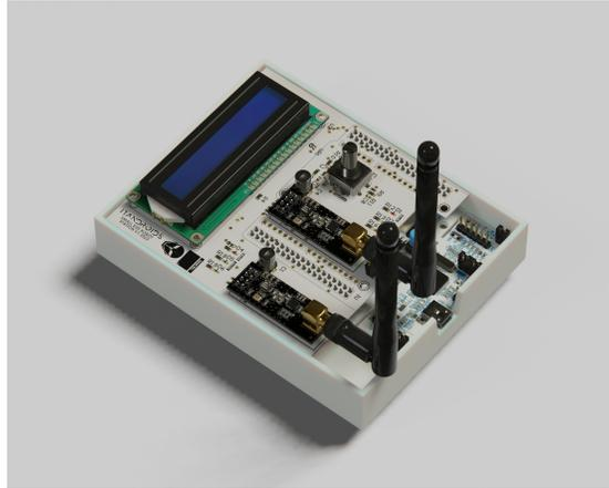
Fig. 1: A rendered image of the Transceiver Station v2 designed in Altium Designer.
