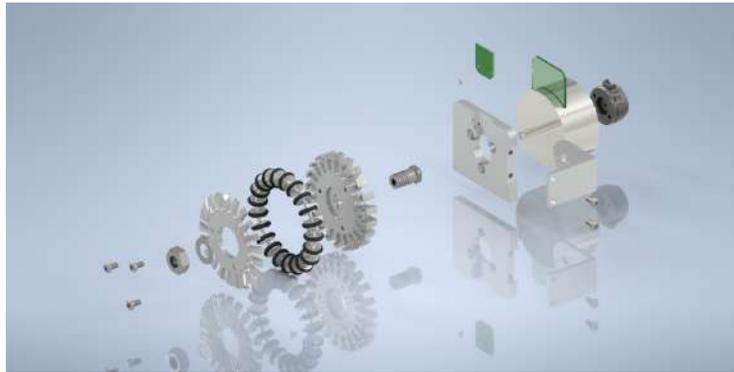
**Fig. 3.** Exploded view of the Transmission Module.
