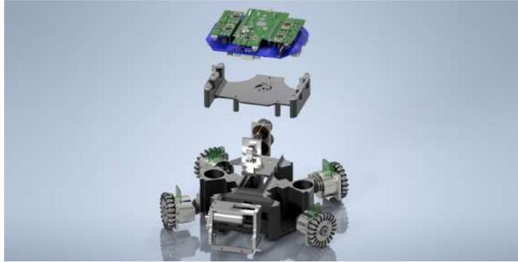
**Fig. 2.** Exploded view of RoboFEI v2025.
