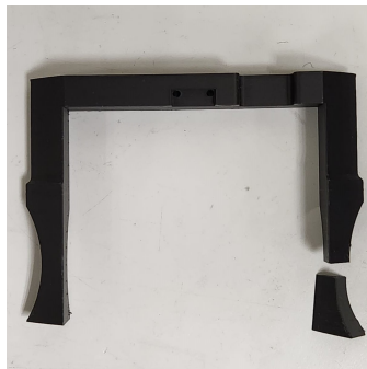
Fig. 9: The front structure with a broken pillar due to collision.
