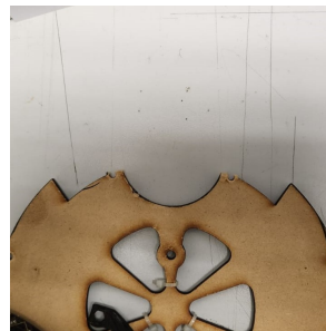
Fig. 2: Top base with a missing section due to worn-out holes.
