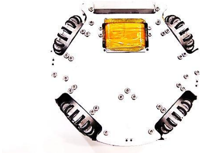
Figure 20: Robot new chassis with added stands' screws.
